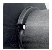
Rope guide for correct winding of the wire rope.
