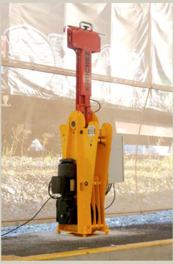
Specific solution developed for a company belonging to a French food industry group for rapidly loading and unloading railway carriages that transport bottles used in the production of natural mineral water. This task was previously carried out manually.
