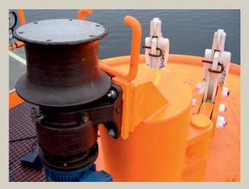
Capstan with foot pedal control. Capacity: 1.5 t. Speed: 25 m/min.
