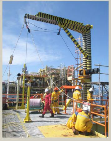
ATEX lifting winch used on an oil platform.
