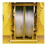
Two independent wire ropes with a breaking load of 1600 kg each (safety coefficient equal to 10).
