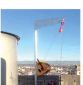
Jib crane with manual winch MANIBOX and wall mounted
