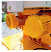
☐ Two independent winches: one ensures the lifting function, the other the fall protection function. Both winches are synchronized.
