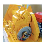
A Reducer - reverser - Brake.
